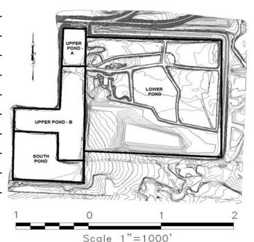
Summarize Overall Condition of Levee Embankments: The overall condition of the perimeter levee embankments is good. Evidence of sloughing or seepage was not observed during the inspection. Empire had plumbing work on-going at the northwest corner of the Upper Pond as of the date of the Inspection.
